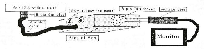
Some dexterity is required with a soldering iron, but other than that it is a fairly easy project to complete. Where noted, part #'s are from Radio Shack or Cardinal Electronics. Two 4-conductor speaker or telephone cables may be used, with a spare conductor to act as the shield connection. I chose to make my own 6-conductor cable with a shield out of scraps I had around the house. Cost: less than \$10.00!
